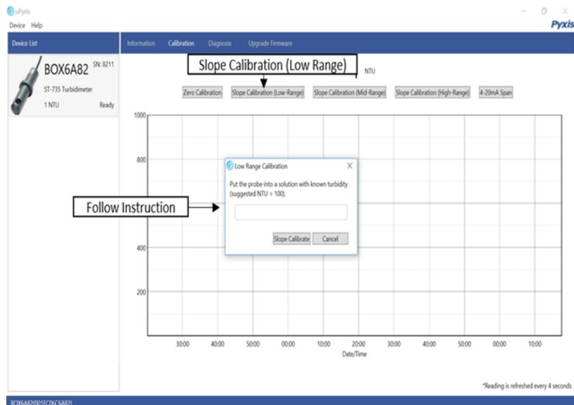
To perform Slope Calibration (Mid Slope), click on **Slope Calibration (Mid Range)**. Then follow the instruction on how to calibrate, then click **Slope Calibration**.
