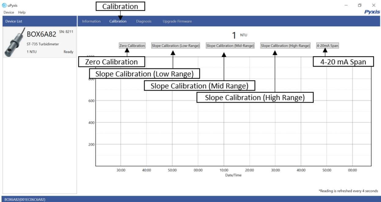
To perform Zero Calibration, click on **Zero Calibration**. Then follow the instruction on how to calibrate, then click **Ok**.
