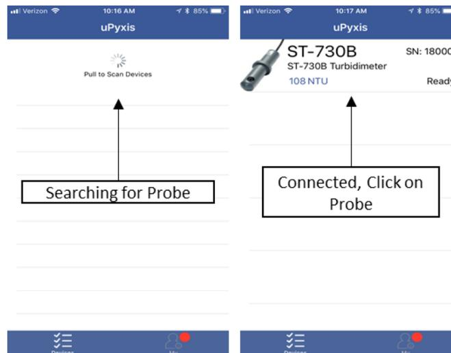
When connected, uPyxis Mobile App will default to the **Calibration** screen. From the Calibration screen you can see the readings and calibrate the ST-730B probe. To perform Zero Calibration, click on **Zero Calibration** and follow the uPyxis app prompts. To perform Slope Calibration, click on **Slope Calibration** and follow the uPyxis app prompts. To perform 4-20 mA Span, click on **4-20 mA Span** and follow the uPyxis app prompts.
