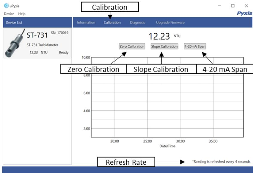
To perform Zero Calibration, click on **Zero Calibration**. Then follow the instruction on how to calibrate, then click **Ok**.
