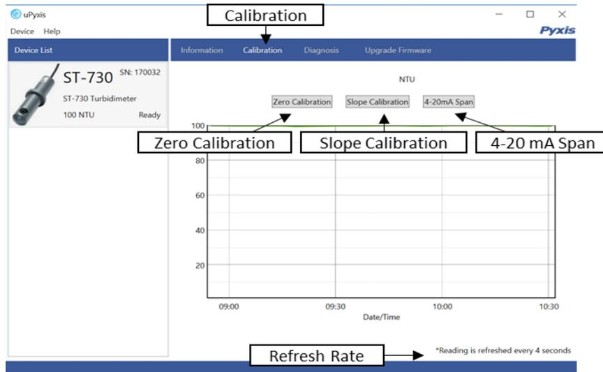
To perform Zero Calibration, click on **Zero Calibration**. Then follow the instruction on how to calibrate, then click **Ok**.
