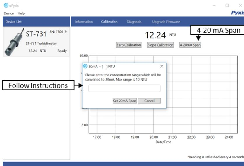
After the device has been calibrated and installation has been completed. To check diagnosis, click on **Diagnosis**. When in the Diagnosis screen you can view the Diagnosis Condition of the device.
