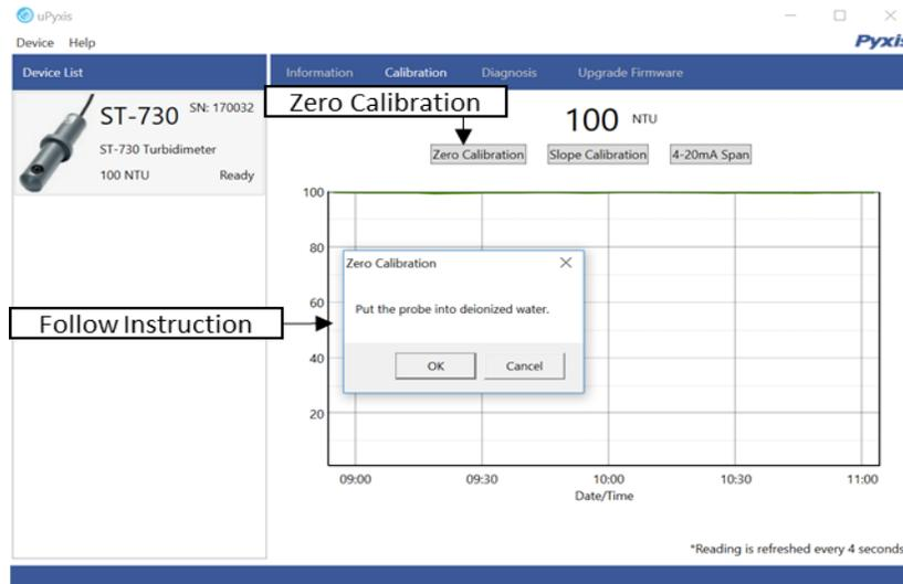
To perform Slope Calibration, click on [Slope Calibration](#). Then follow the instruction on how to calibrate, then click [Slope Calibration](#).
