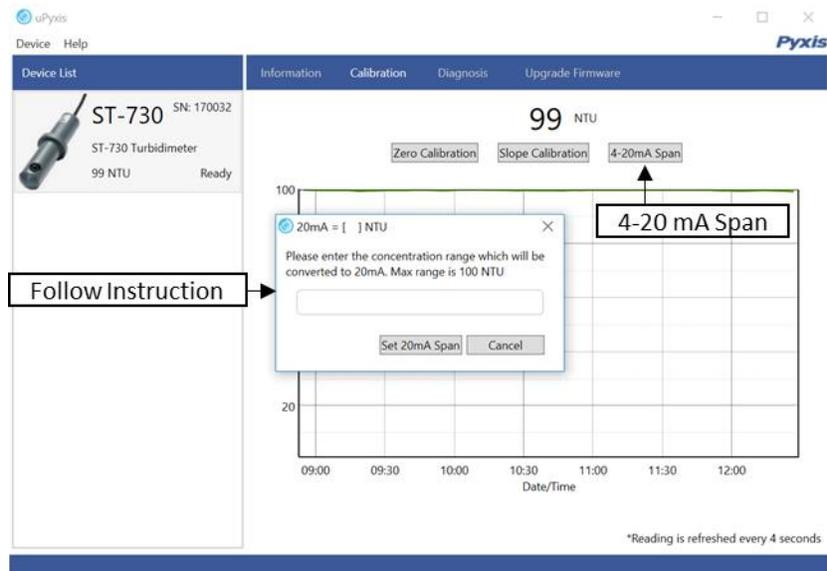
After the device has been calibrated and installation has been completed. To check diagnosis, click on **Diagnosis**. When in the Diagnosis screen you can view the Diagnosis Condition of the device.
