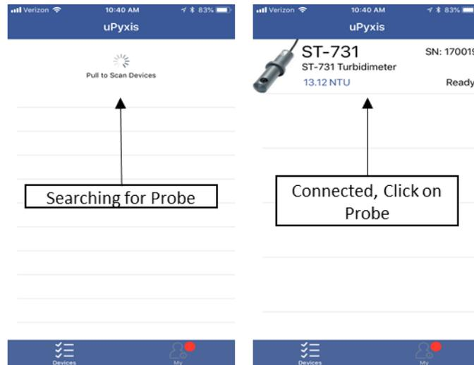
When connected, the uPyxis Mobile App will default to the **Calibration** screen. From the Calibration screen you can see the readings and calibrate the ST-731 probe. To perform Zero Calibration, click on **Zero Calibration** and follow the uPyxis app prompts. To perform Slope Calibration, click on **Slope Calibration** and follow the uPyxis app prompts. To perform 4-20 mA Span, click on **4-20 mA Span** and follow the uPyxis app prompts.
