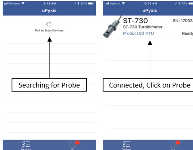
When connected, the uPyxis Mobile App will default to the **Calibration** screen. From the Calibration screen you can see the readings and calibrate the ST-730SS probe. To perform Zero Calibration, click on **Zero Calibration** and follow the uPyxis app prompts. To perform Slope Calibration, click on **Slope Calibration** and follow the uPyxis app prompts. To perform 4-20 mA Span, click on **4-20 mA Span** and follow the uPyxis app prompts.
