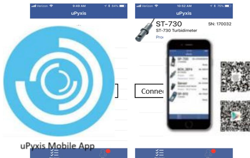
When connected, uPyxis Mobile App will default to the **Calibration** screen. From the Calibration screen you can see the readings and calibrate the ST-730 probe. To perform Zero Calibration, click on **Zero Calibration** and follow the uPyxis app prompts. To perform Slope Calibration, click on **Slope Calibration** and follow the uPyxis app prompts. To perform 4-20 mA Span, click on **4-20 mA Span** and follow the uPyxis app prompts.
